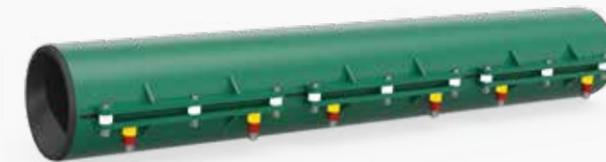
Specially designed Wear Compensation Stator design allows to control and regulate the efficiency of Progressive Cavity Pumps for an extended period. It uses spacers of engineered lengths to maintain even interference throughout the length of rotor and stator.
